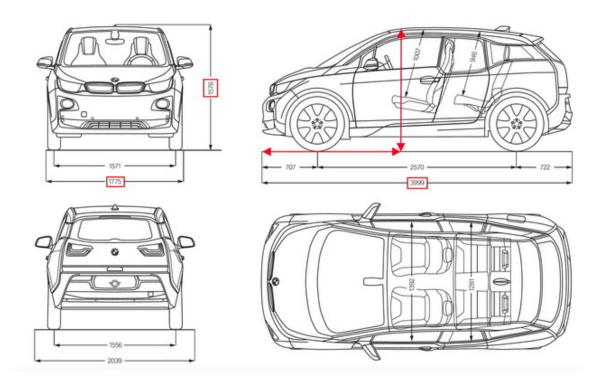
As the height is concerned, the car to be hauled should not exceed 62" (see vertical red line) at a distance of approx. 70.5" from its front end (see horizontal red line) and should not get higher from there towards its rear end. The overall length is 157.4" and the width about 70" with mirrors folded (garage accommodates a little bit more in either direction).
